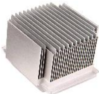
Socket processor with passive heat sink (no cooling fan)
