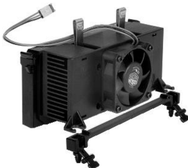
Slot processor with active heat sink (cooling fan)
